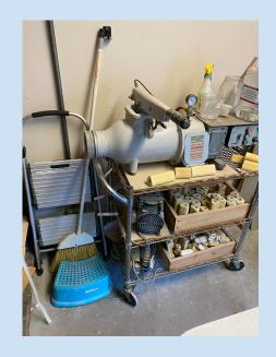
Pugger- used to mix, recondition scrap clay, and extrude prepped clay for new projects.
